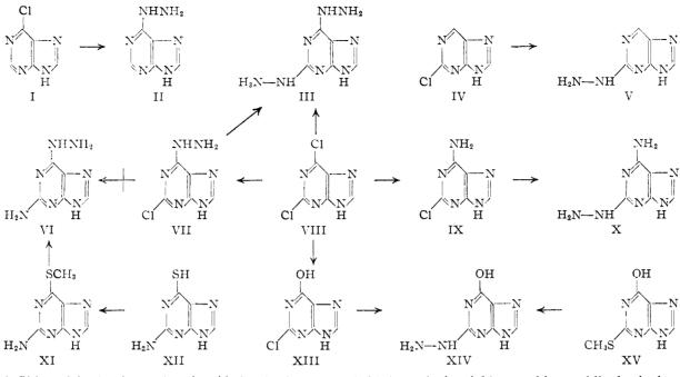
2-Chloro-6-hydrazinopurine  $(VII)^{15}$  is obtained at room temperature and it is necessary to heat the solution of 2,6-dichloropurine in anhydrous hydrazine to 80° for 12 hours to obtain 2,6-dihydrazinopurine (III).
